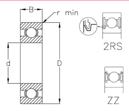
B = 5 d = 17 D = 26 Dynamic load C (kN) = 2.81 Max rpm greased = 24000 Max rpm oil lubricated = 28000 r min = 0.3 Static load C0 (kN) = 1.72
